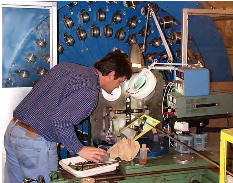
64-strand cabling machine at Berkeley
